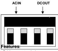
Quick connect terminals 1.0 Amp Supply Current Power Adapter Input: 20~30V AC
