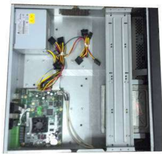
Figure 3-45 Put bracket back
