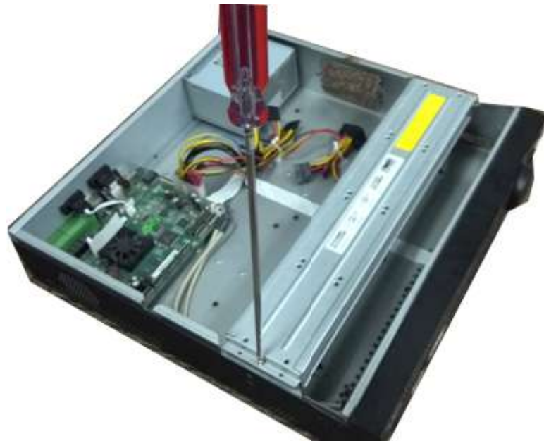
Figure 3-37 Open the top cover
