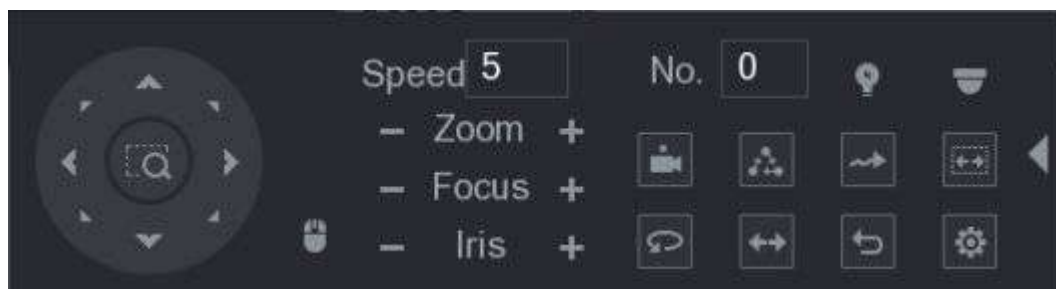
Figure 5-53 Expanded PTZ control panel
