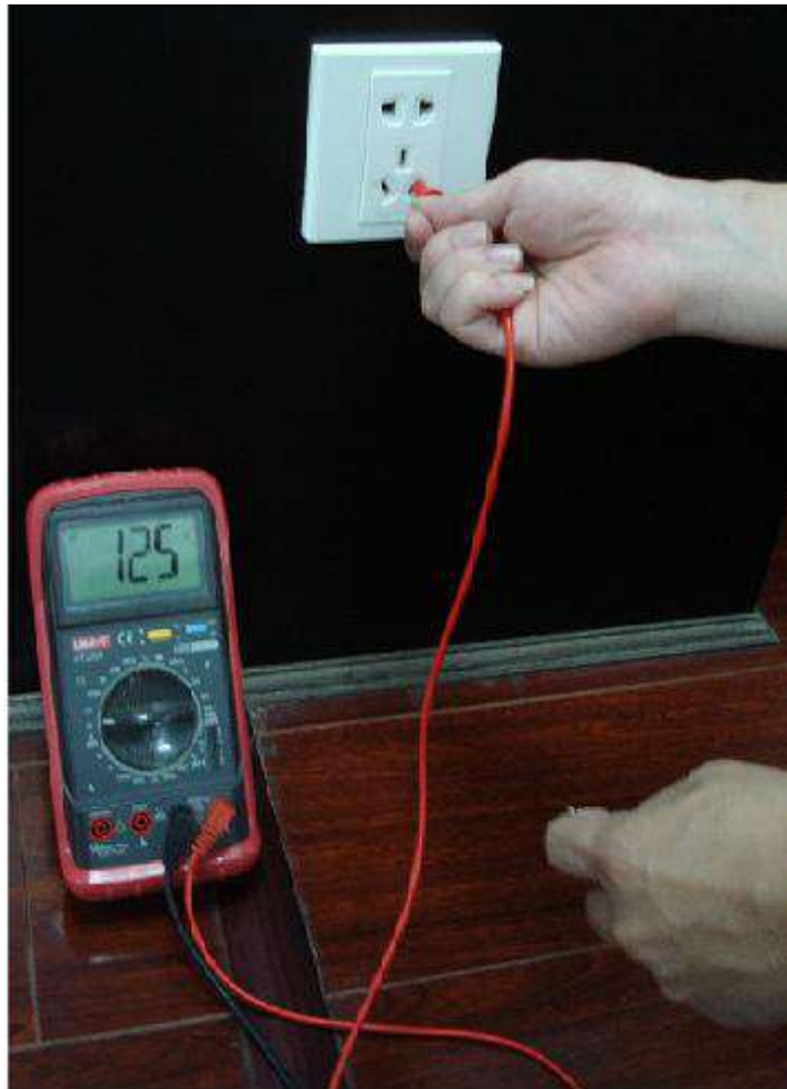
Appendix Figure 7-6 Check live cable connection
