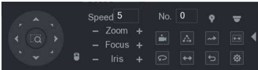
Figure 5-53 Expanded PTZ control panel
