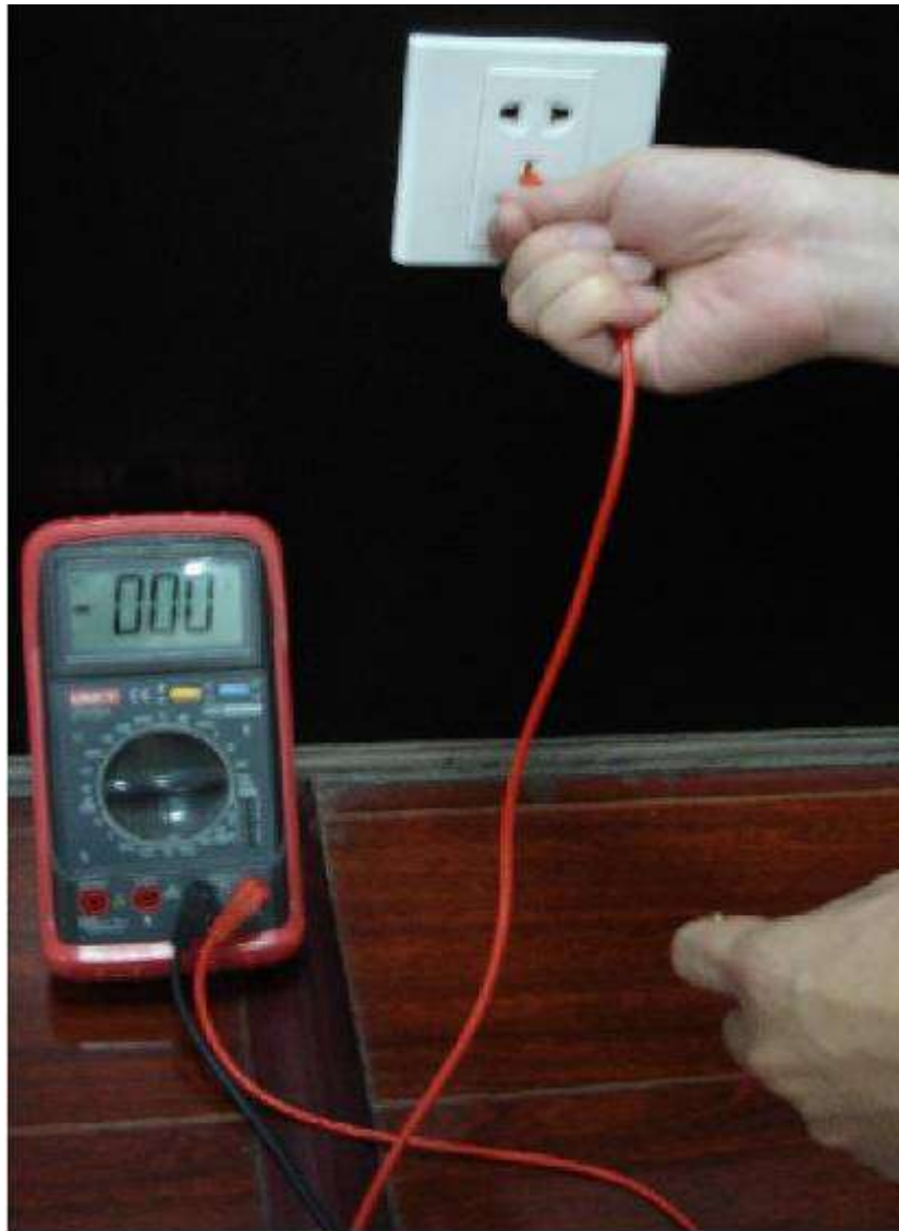
Appendix Figure 7-5 Check earth cable connection
