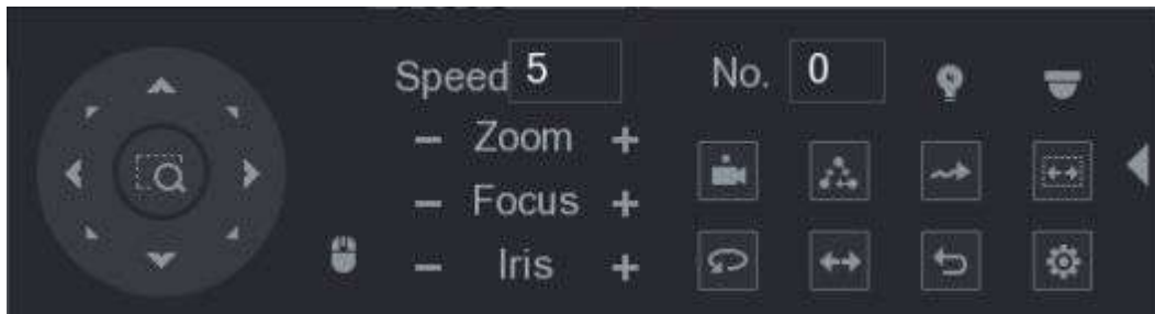
Figure 5-58 Expanded PTZ control panel
