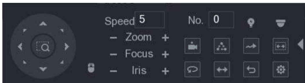
Figure 5-53 Expanded PTZ control panel
