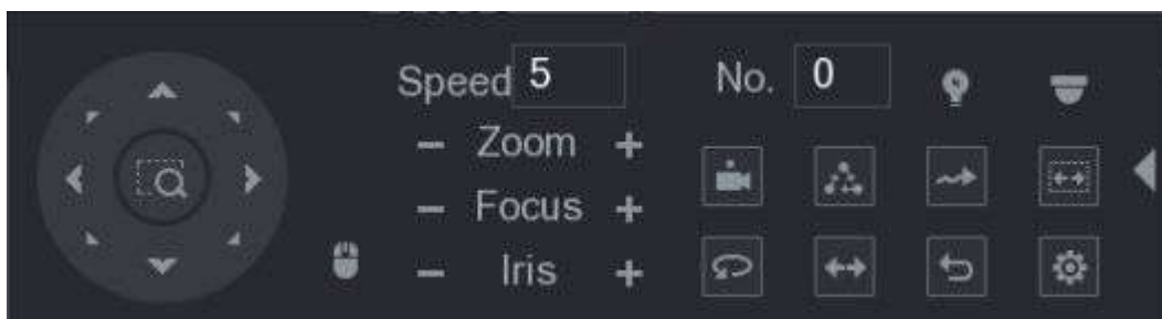
Figure 5-53 Expanded PTZ control panel
