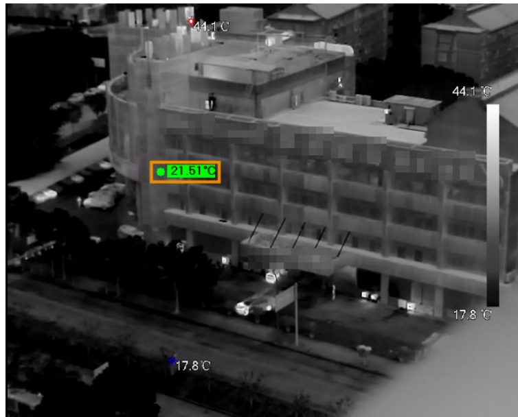
Figure 4-6 Real-time spot temperature measurement
