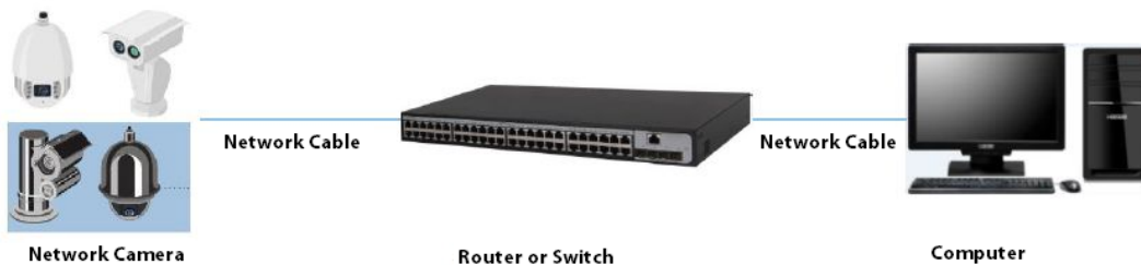
Figure 1-2 Connected through network router or switch
