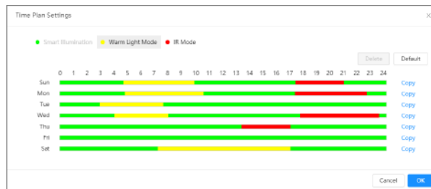
Figure 6-12 Time plan settings
