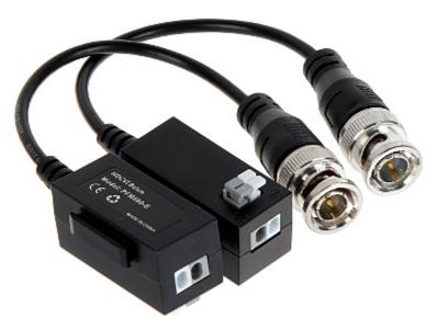
PFM800-E is designed for the transmission of video signals over a twisted pair cable. The equipment adapts the impedance of the 75  $\Omega$  coaxial cable to the impedance of the symmetrical cable, which guarantees the transmission of the video signal at a distance of up to 400m @ 720p (category 5 twisted pair cable) and eliminates asymmetric interference .
