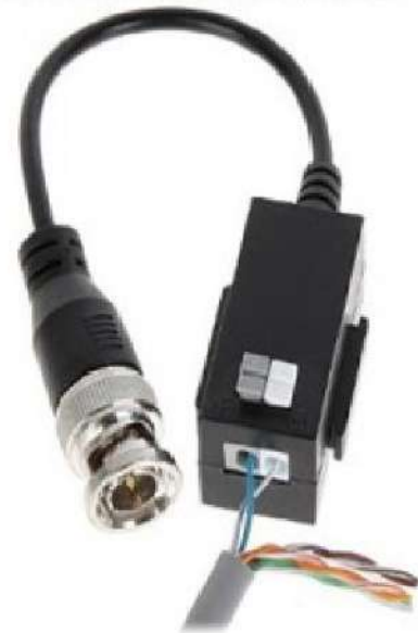
Connecting the twisted pair cable to the transformer:
