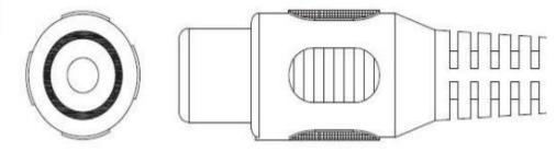
Can be connected via RCA connector to a camera (harness connector) or to a recorder (rear panel connector, illustrative panel image)
