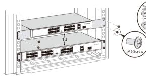
1. Install 4 floating screws on the front hole bar of the cabinet, 2 on each side.
