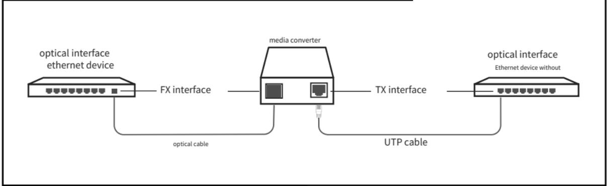
Scenario 2: Connecting a device without an optical interface
