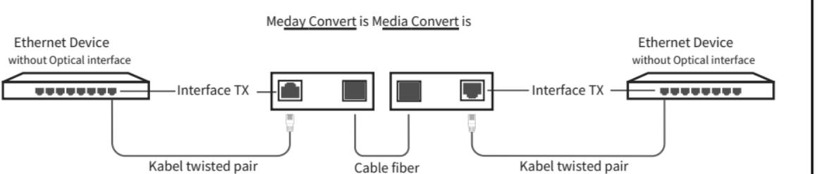
Scenario 1: Connecting devices with and without optical interfaces
