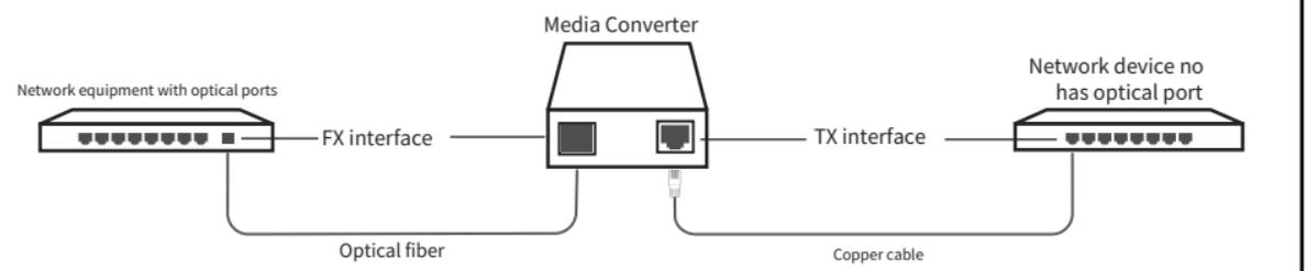
Scenario 2: Connecting a device without an optical port
