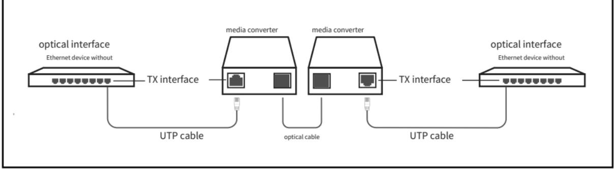
Model 1: Connect devices using and without using fiber-optic cables.
