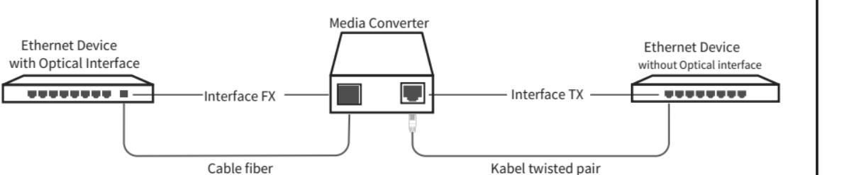
Scenario 2: Connecting a device without an Optical Interface
