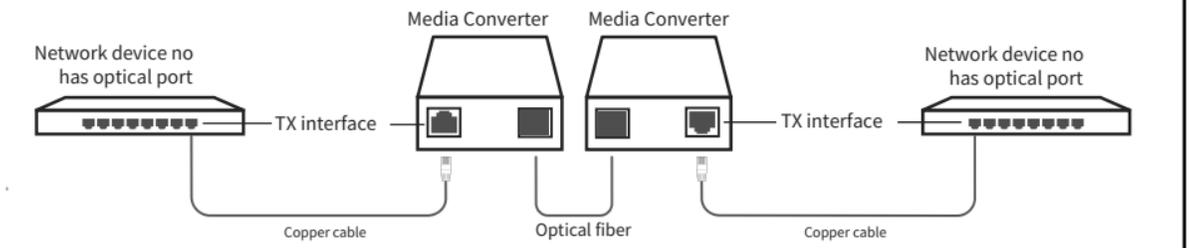
Scenario 1: Connecting devices with and without Optical Interface
