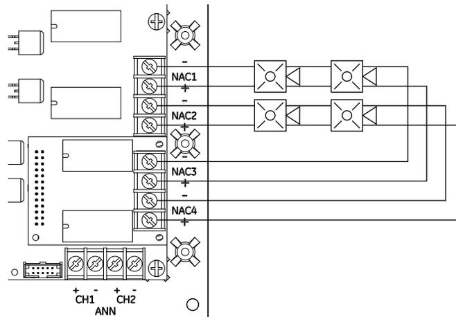
**Figura 36: Circuito de anunciador remoto redundante Clase B con tarjeta SA-CLA**
